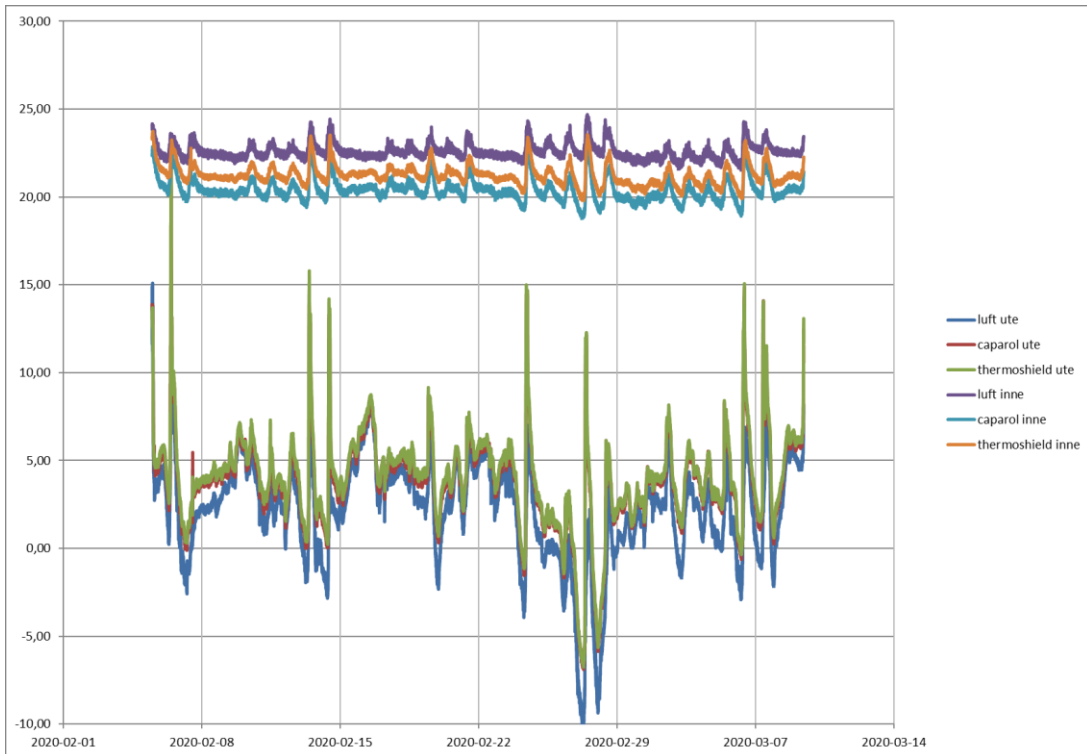
Measured temperatures for both wall panels from 05/02/2020 to 09/03/2020
