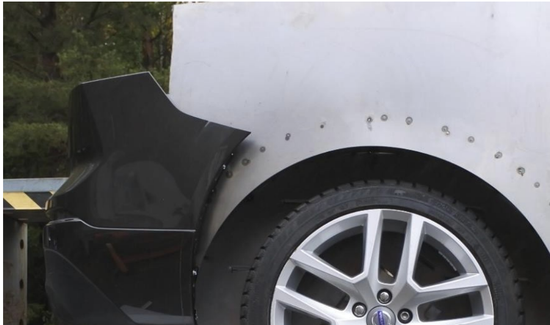
Figure 1. Test rig for generating stone chips. Shown here without a splash guard.
