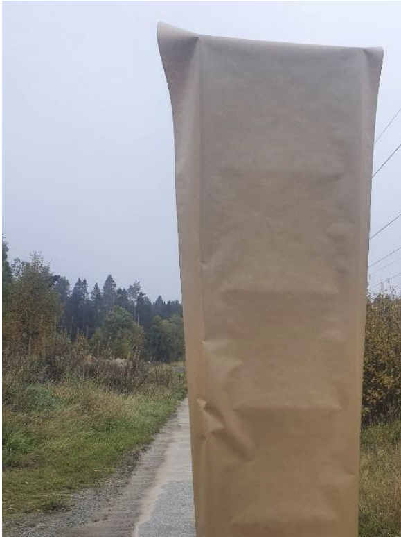
Figure 2. Kraft paper mounted on the stand for stone chip detection.
