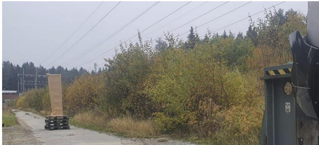
Figure 4. Test set-up with the stand placed 17 m from the wheels' contact point.
